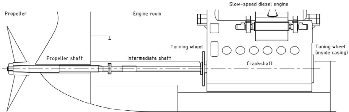
**Fig. 1** Typical merchant ship propulsion plant (Note: bearings omitted in order to maintain clarity)
