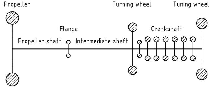
**Fig. 2** Torsional vibration scheme of the propulsion system
