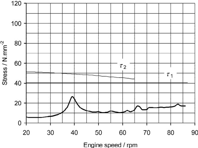
Fig. 5 Crankshaft stress response for the C-2 case
