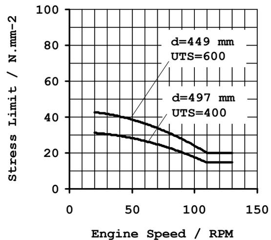
Figure 3. Permissible stress limits for the propeller shaft
