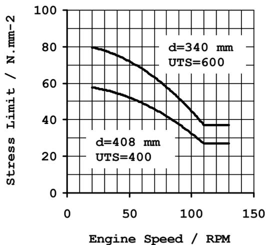
Figure 2. Permissible stress limits for the intermediate shaft
