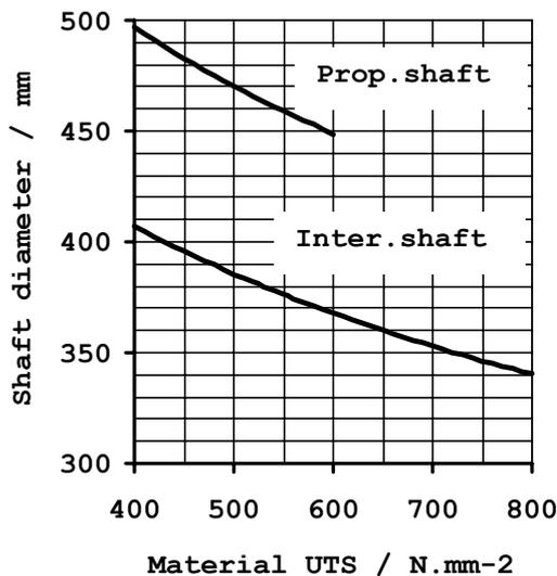
Figure 1. Material influence on the shaft minimum diameters
