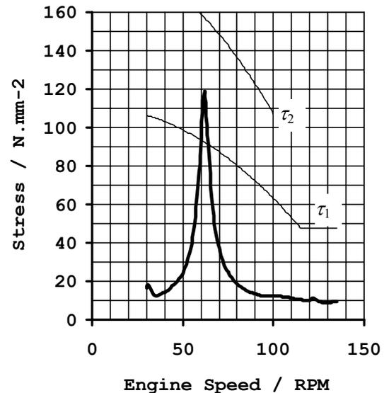
Figure 7. Torsional stress in intermediate shaft for final design
